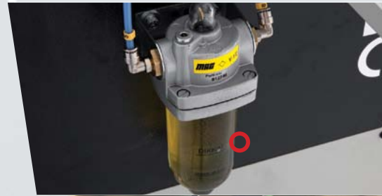
Cutting oil spray system
