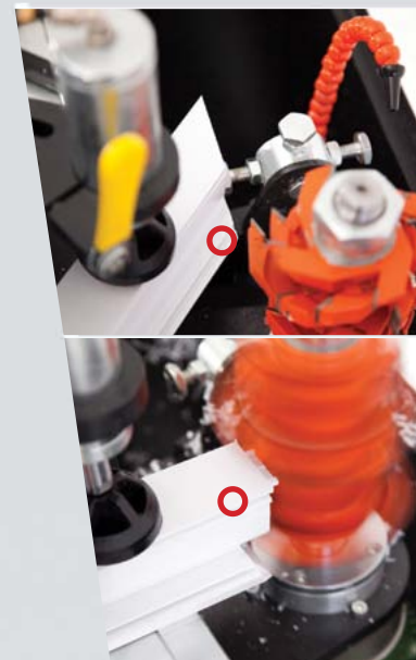
End milling operations
